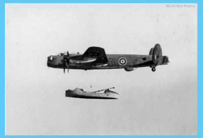
the sea, water immersion switches would initiate the firing of rockets which disengaged the parachutes to take them clear of the craft.
